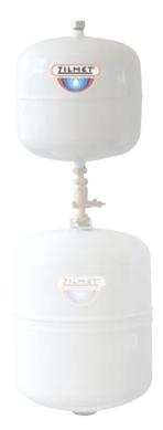
According to our experience and the reviewing of different international regulations on solar energy an additional tank is recommended when the fluid volume between the collector and the expansion vessel is approx 50% or less than the 'wet' side volume (between the expanded diaphragm and the vessel inlet). This approach is covered by the European Directive VDI 6002.
